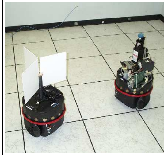
FIGURE 1.1. Two robots exploring the environment employing cooperative localization.
