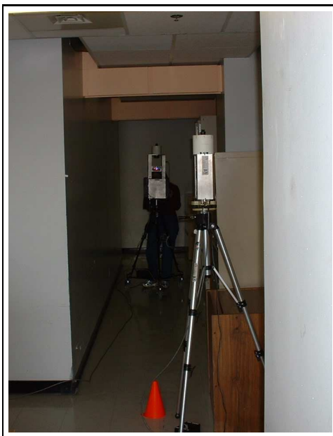
FIGURE 1.3. The system consists of two stations mounted on tripods. One tripod is positioned on a fixed location and acts as a reference point. The second tripod is on wheels and carries two sensors, one localization sensor that is able to infer the position of the moving tripod relative to the reference point and a laser range finder that is used in order to map the distance to various objects (walls, corners, etc.).
