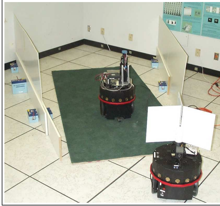
FIGURE B.1. Measuring the odometry error on carpet.
