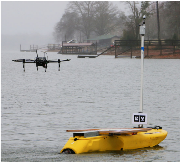
FIGURE 1 A view of the UAV-ASV marsupial system where the UAV follows the ASV at a safe distance during field trials. ASV, Autonomous Surface Vehicle; UAV, Unmanned Aerial Vehicle [Color figure can be viewed at wileyonlinelibrary.com ]
