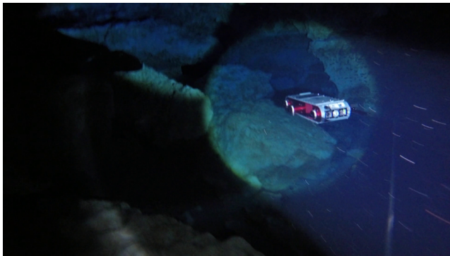
Fig. 6. Aqua2 AUV navigating inside the Ginnie Ballroom, FL. A diver plays the role of the distal observer with a GoPro camera (Joshi et al., 2022) and a light illuminating the AUV and the surroundings.
