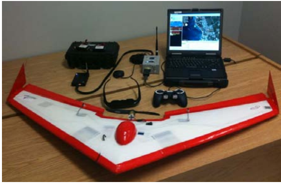
Fig. 4. The Unicorn is a fixed-wing UAV with an on-board autopilot microprocessor and a gimbal-mounted camera.
