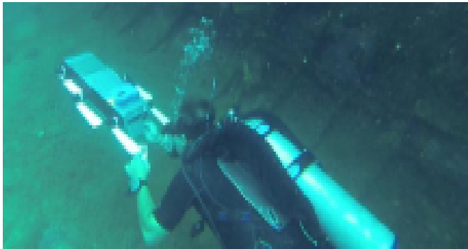
Figure 1. A diver controlling the robot using a cue-card
