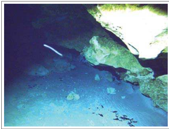
Fig. 8. A small particle reflecting back at high speed generating a blurry streak. In addition light reflecting back from a nearby surface completely saturates the camera.
