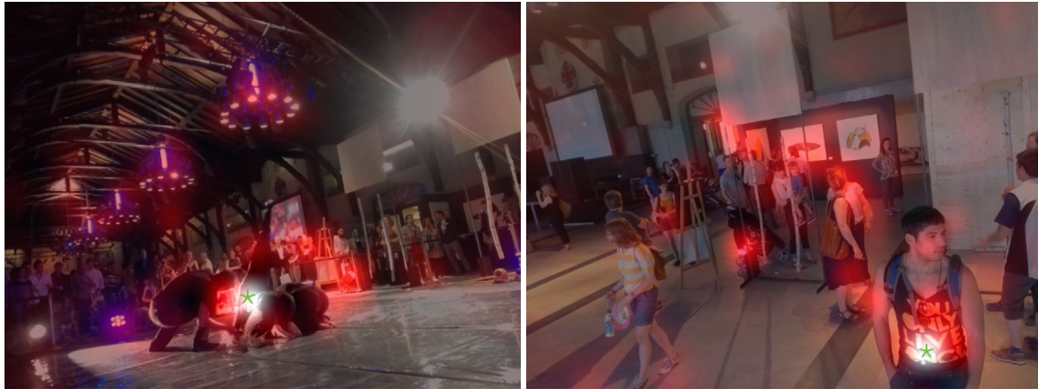
Fig. 23. Examples of interesting observations captured by the curiosity module, mounted on Tryphon. The interesting parts of the scene are highlighted with red color, and the most interesting part of the scene is marked with the white blob overlaid on real images. On the left we see the curiosity module fixated on the performers as they do their routine, and on the right we see the module being interested in an audience's eye t-shirt. (For interpretation of the references to color in this figure legend, the reader is referred to the web version of this article.)
