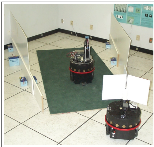
Figure 6.1: Measuring the odometry error on carpet.
