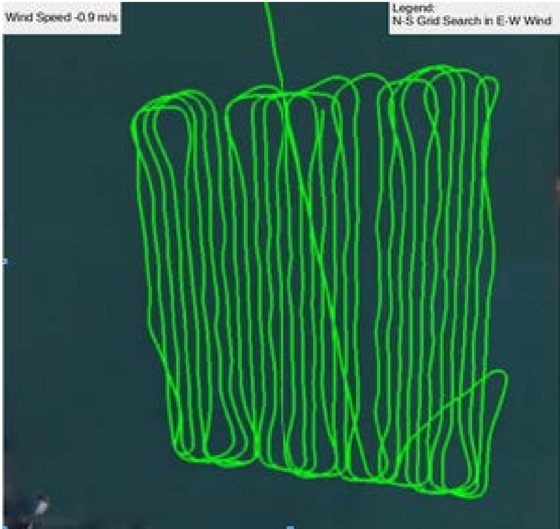
Figure 3.8: Trajectory for grid search conducted by a single Jetyak with tuned PID coefficients.
