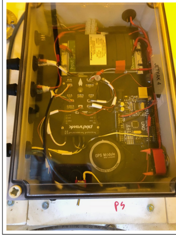
Figure A.5: Electronics box of the ASV, which contains controllers and sensors, including GPS and Arduino. Each of the components can be a source of noise.
