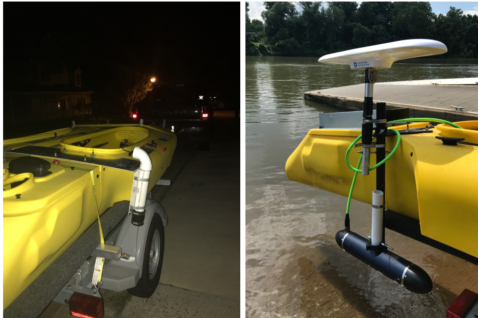
(a) Brute force early mounting system. (b) Modular, rigid, and adjustable mounting system.
