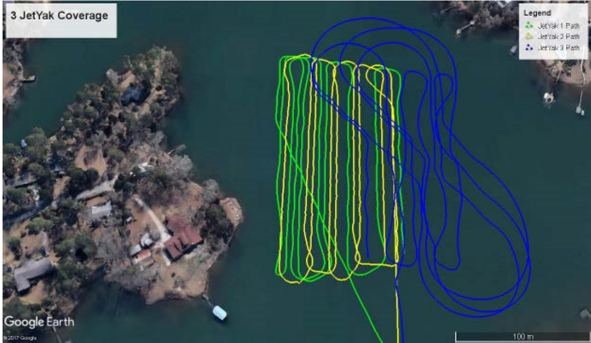
Figure 3.10: Trajectories for three JetYaks searching their respective areas of responsibility according to mission resulting from implementation of our multi-robot coverage algorithm for Dubins vehicles.
