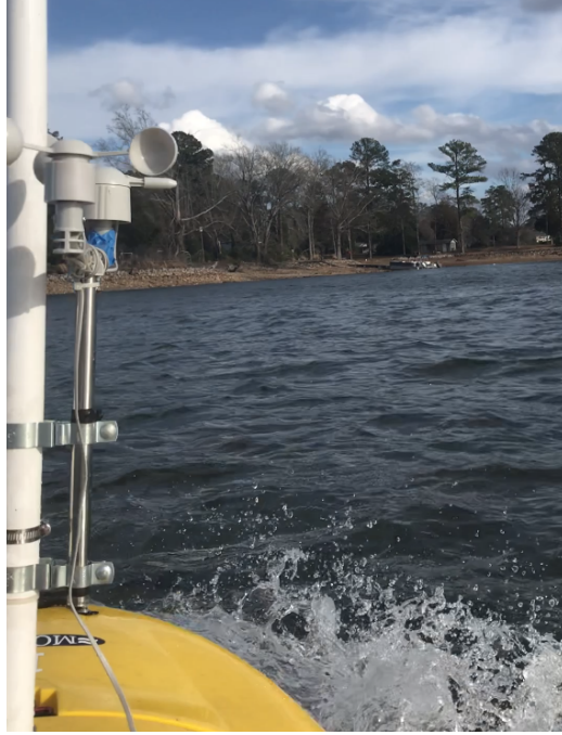
Figure 6.1: UofSC’s custom-made ASV gathering wind data with anemometer and wind vane in windy conditions on Lake Murray, SC.
