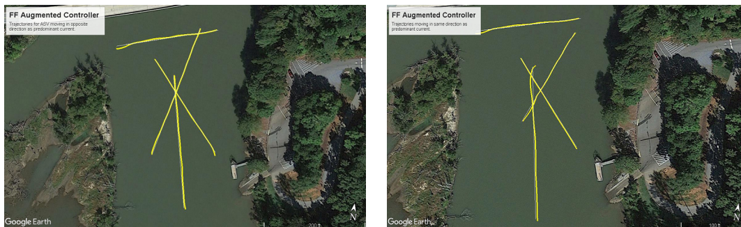
Figure 6.18: Augmented Pixhawk way-point navigator tracking in slow currents with the ASV travelling mainly (a) against the predominant direction of the current; (b) with the predominant direction of the current – white line: target trajectory, yellow line: actual executed trajectory.
