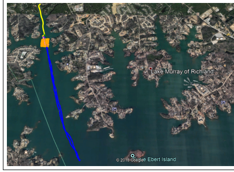
Figure A.7: GPS trace-path of deployed ASV on Lake Murray to evaluate communication between BS and ASV in LOS. Yellow traces represent low latency, orange represent ASV executing way-point missions, and blue traces evaluate the quality of communication and range limitation.
