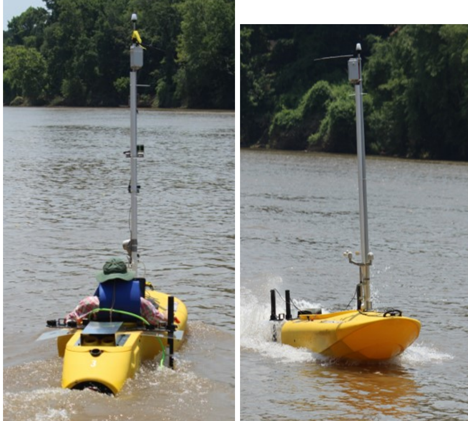
(a) Supervised Jetyak 3 with Ping (b) Unsupervised Jetyak with an- DSP 3D sidescan imaging trans-chor light, communication hub, ducer, anchor light, communication anemometer, 2 surface current and hub, lidar, GPS, stereo camera, and depth sonar sensors deployed. monocular camera deployed. Engine wave guard and sensor splash guards are also installed and functioning.
