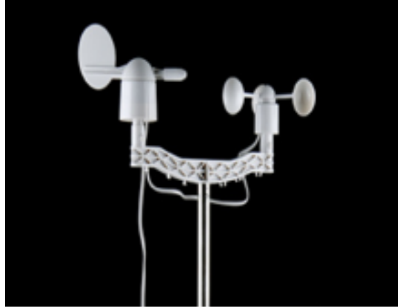
Figure 4.2: SparkFun anemometer mast mount for wind speed and direction measurement.
