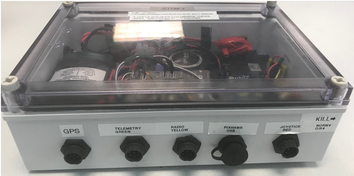
Figure 3.6: Pixhawk Box with power conditioner, Pixhawk PX4, Arduino Uno, GPS, joystick outputs, remote control interface, MAVLink -MAVROS node proxy inputs/outputs collocated.
