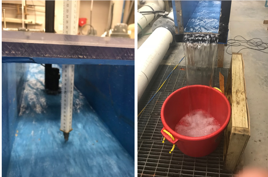
(a) Measuring the cross section of the water flow on the flow table. (b) Measuring the time the flow takes to fill a known volume.
