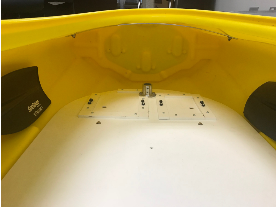
Figure 3.2: Front portion of marine grade starboard sub-floor with footings for battery, control box, as well as topside and anchor mast ports installed.
