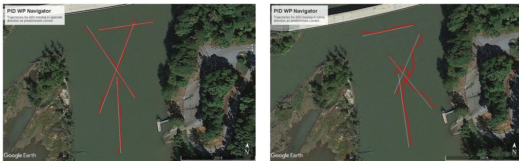
Figure 6.17: Pixhawk PID controlled way-point navigator tracking in slow currents with the ASV travelling mainly (a) against the predominant direction of the current; (b) with the predominant direction of the current – white line: target trajectory, red line: actual executed trajectory.
