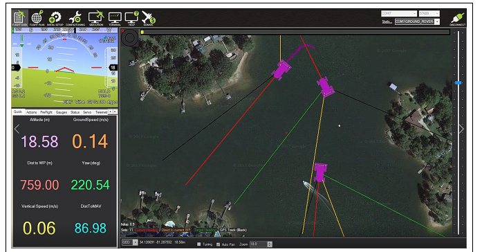
Fig. 4. Live monitoring of 3 ASVs deployed at Lake Murray. Data was collected from various experiments where each ASV was connected to a separate GCS operating on different Net IDs, and this illustration where all were monitored by a single GCS. All BSs were connected to laptops stationed at shore running Mission Planner software for monitoring and data collection.
