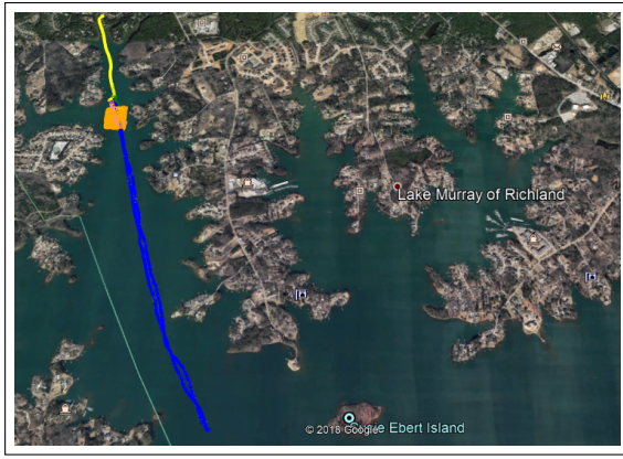
Fig. 7. GPS trace-path of deployed ASV on Lake Murray to evaluate communication between BS and ASV in LOS. Yellow traces represent low latency, orange represent ASV executing way-point missions, and blue traces evaluate the quality of communication and range limitation.
