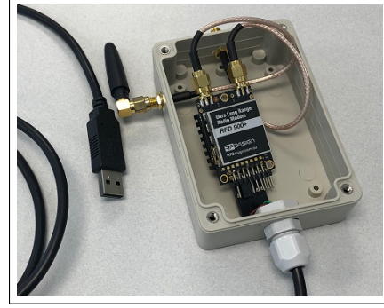
Fig. 2. RFD900+ modem installed in a waterproof box, connected by FTDI cable.
