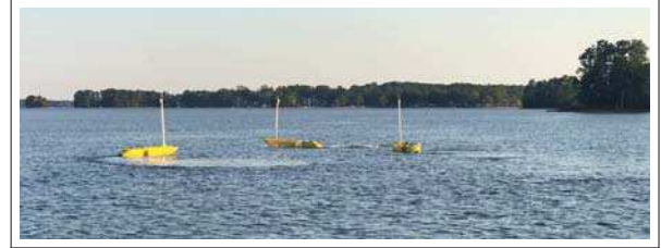
Fig. 1. Three autonomous surface vehicles during coverage experiments at Lake Murray, SC, USA.
