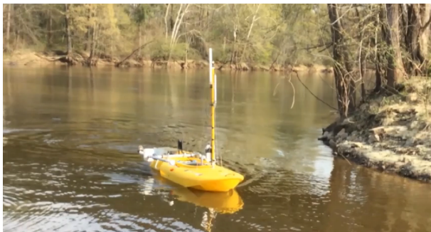
Fig. 10. Autonomous Surface Vehicle (ASV) based on the Mokai Eclipse platform.
