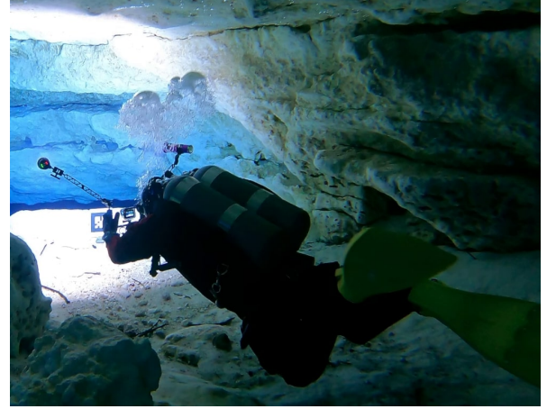
Fig. 1: GoPro setup deployed inside a cave, Ginnie Springs, FL. A fiducial tag can be seen, used for estimating ground truth.
