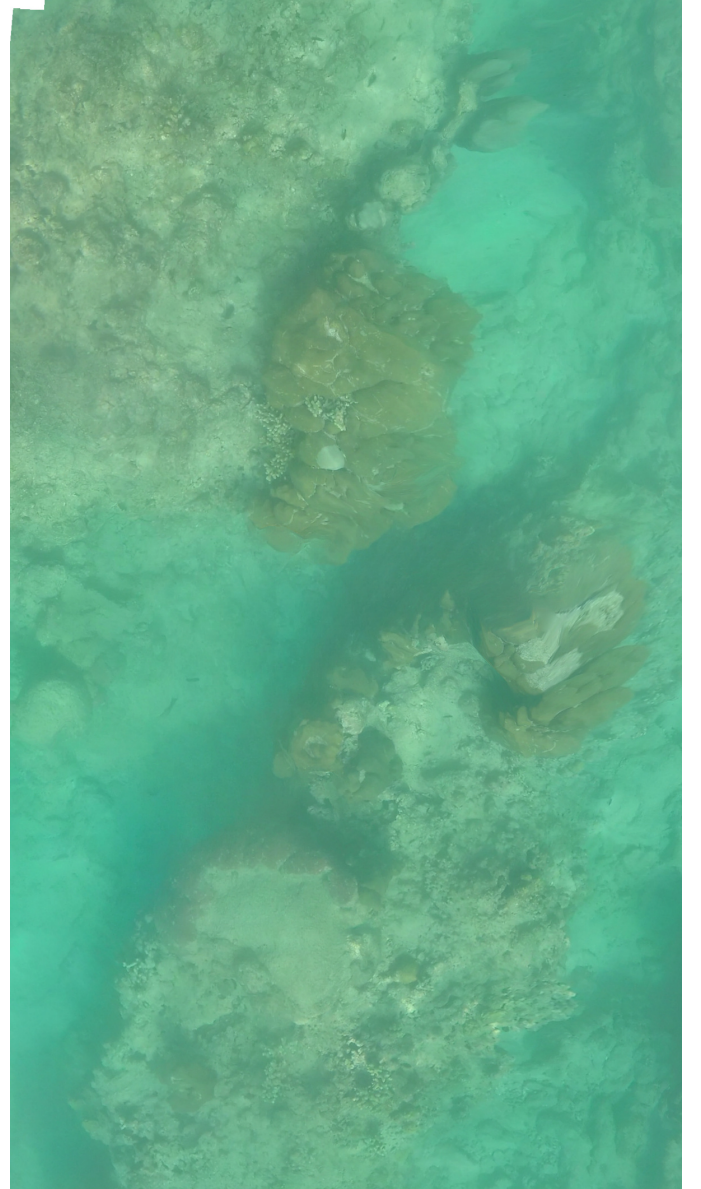
Figure 8: Mosaic developed using 27 images captured from ASV over coral heads. The mosaic is cropped to fit the column width.
