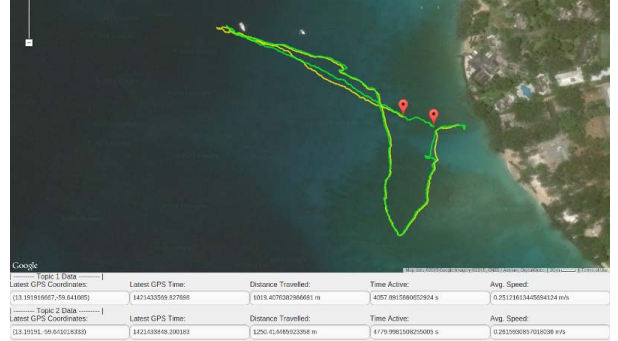
Figure 5. The GPS trails of two drift nodes as they moved off the coast of Barbados. During the experiment different behaviors were studied. Free drifting; constrained drifting near an anchor point; moving a single node and towing the other; moving both nodes with fixed orientation and at a fixed distance between them.
