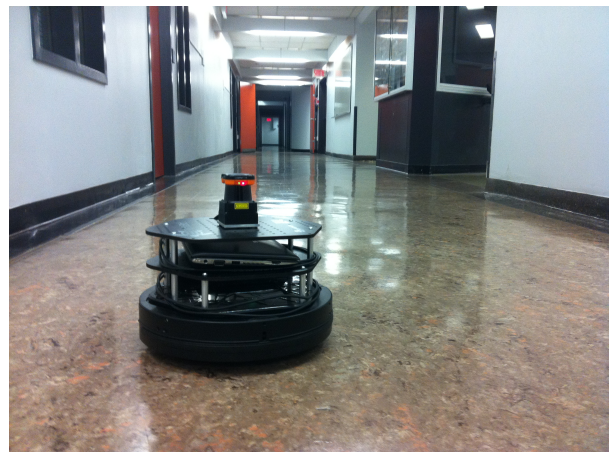
Figure 1. Our main robotic platform, a TurtleBot 2, is equipped with a Hokuyo laser range-finder used for navigation. Several experiments performed with this configuration validate the Ear-based exploration, the construction of the hybrid Metric/Topological map, and the heuristic path planning.
